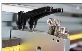
Fine pressure adjustment (according to the types of material)
