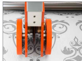
Single lengthwise rotary crush cutter (twin cutters optional)
