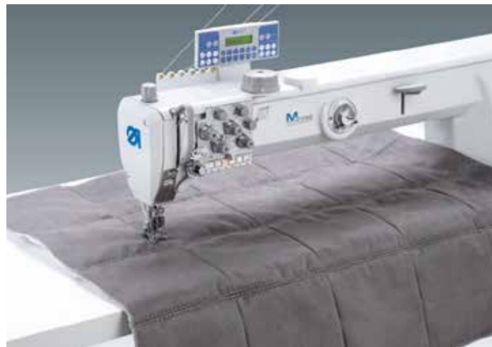
Sewing device E724/12 for topstitching large, voluminous upholstery parts.
