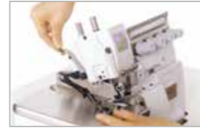
Easy to handle pressure feed with lever
