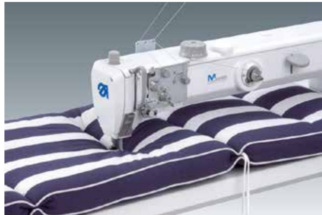
With shuttle foot for topstitching seat covers.
