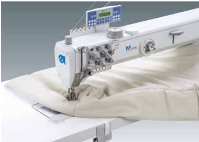
Sewing equipment E724/12 for two-needle decorative seams on particularly large padded leather upholstery covers.
