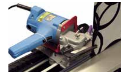
Cutter with big diameter 100mm - widia counterblade and sharpening device.
