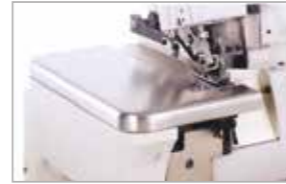
Cover plate combined with side panels, which can be opened together
