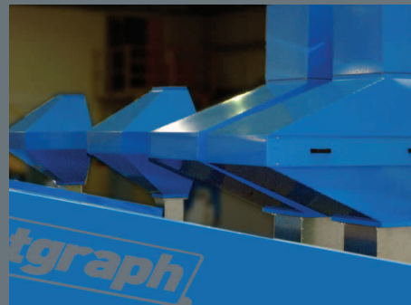
Inlet air filter stacks
