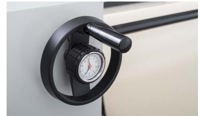
Felt tensioning adjustment with pressure gauge
