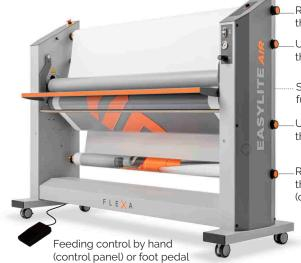
Rewinding clutched shaft for adjusting the tension of the liner
