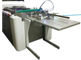
**SHEET FEEDER**Feed width up to 52 cm / 20"
