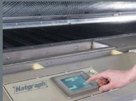
Touch Screen PLC Control
