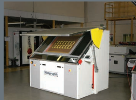
Pneumatic lifting of frames
