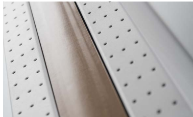
Suction plate to perfectly center the media to be welded
