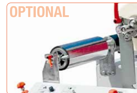
Hot stamp: Multifunctional devise that allows varnish, holograms finishing as well as gold, silver and wide variety of metallic colours foiling effect.
