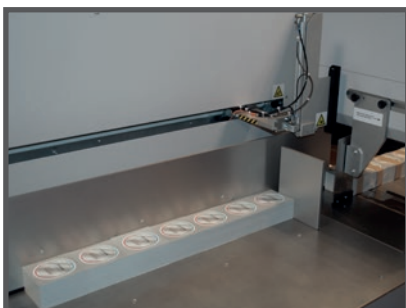
1. Manual insertion and alignment of product piles
