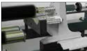
Mobile tailstock assembly for smaller shafts (optional)
