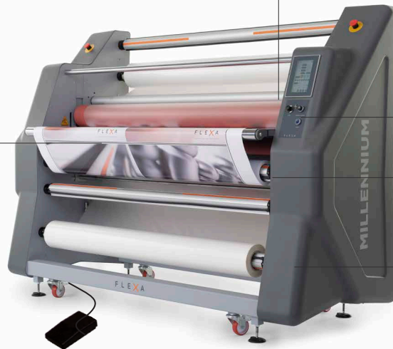
Feeding control by hand (control panel) or foot pedal (hand free operation)
