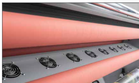
Rear traction rollers with forced cooling system for encapsulation, heat laminated prints and application of double-adhesive
