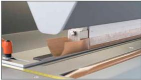
Welding bars covered by protective teflon tape (antigloss teflon optional) preventing the welded media from sticking to the bars
