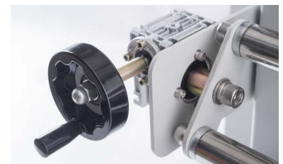
Fabric tensioning adjustment
