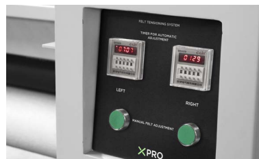
Felt belt automatic tracking system
