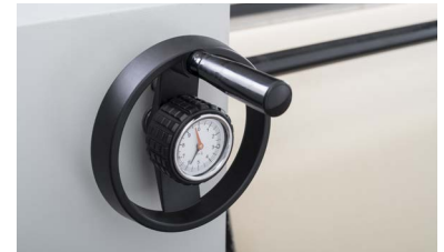
Felt tensioning adjustment with pressure gauge
